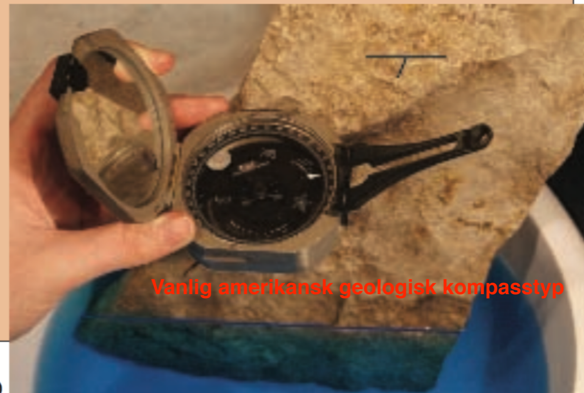
FIGURE 11.6 (a) We use strike and dip to measure the orientation of planar structures such as these tilted beds. The strike is the compass angle between the strike line (an imaginary horizontal line on the plane) and true north. The dip is the angle between the strike line and the dip line (an imaginary line parallel to the steepest slope on the plane) as measured in a vertical plane. Note that the strike line and the dip line are perpendicular to one another. (b) On a map, the line segment represents the strike direction, while the tick on the segment represents the dip direction. The number indicates the dip angle as measured in degrees. (c) To specify the orientation of a line, we use plunge and bearing. The plunge is the angle between the line and horizontal as measured in a vertical plane, whereas the bearing is the compass orientation of the line. (d) To illustrate the concept of strike, a geologist is holding a Brunton compass, a special compass that includes a clinometer, against a slab of rock that has been partially submerged in a basin of water. The surface of the compass is horizontal—meaning it is parallel to the surface of the water—so the edge of the compass in contact with the slab is a strike line.
